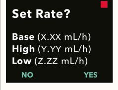
Adjust Base rate-press Next. It will go through High rate and Low rate, adjust and press next as appropriate
